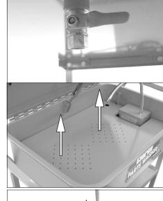
2. Slide the filter holder up from the pump as shown.
