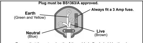
Ensure that the outer sheath of the cable is firmly held by the clamp
